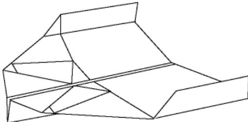
The Bulldog has a compact nose section that makes it very stable by keeping the center of gravity forward. It flies well indoors or in very light breezes outdoors.
