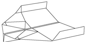
Fold the wings down along fold lines 7 and the winglets up along fold lines 8. Add wing dihedral by tilting the wings up slightly away from the fuselage. The wings will have a slight "V" shape when viewed from the front. You are ready to fly!
